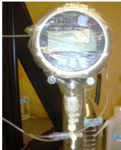
Figure A.1.6. Pressure transducer with open valve.
